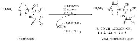
The process of the reaction was monitored by TLC with an eluent of ethyl acetate/petroleum ether (2/1, v/v). Infrared spectra were measured with a Nicolet Nexus FTIR 670. The position of acylation in enzymatically prepared thiamphenicol esters was
